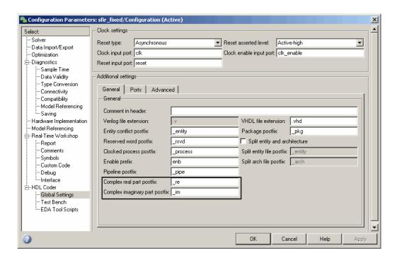
The **Complex real part postfix** option (and the corresponding ComplexRealPostfix CLI property) specifies a string to be appended to the names generated for the real part of complex signals. The default postfix is '\_re'. See also "Complex real part postfix".
