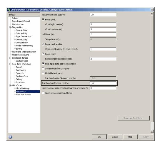
If you generate test bench code via the makeholtb function, use the Testbenchreferencepostfix property (see TestBenchReferencePostFix in the in the Simulink HDL Coder documentation) to specify the postfix string.
