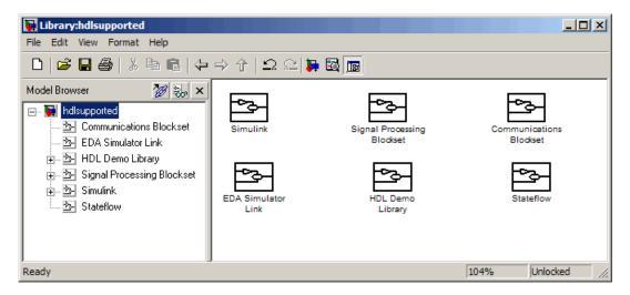
The set of supported blocks will change in future releases of the coder. To keep the hdlsupported.mdl current, you should rebuild the library each time you install a new release. See "Supported Blocks Library" in the Simulink® HDL Coder<sup>TM</sup> documentation for further information.
